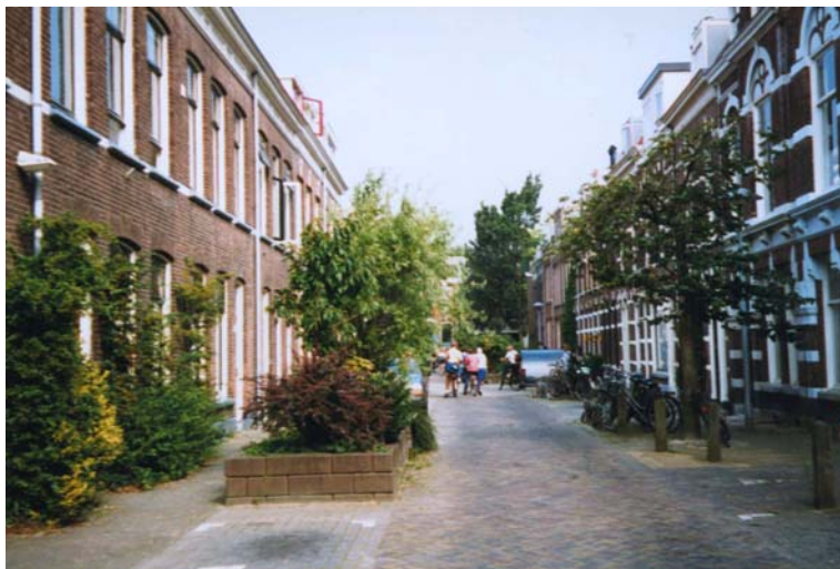
A typical Woonerf (Homezone) in Utrecht, The Netherlands, with shared surface, raised beds and street trees, bike rails and parking bays
